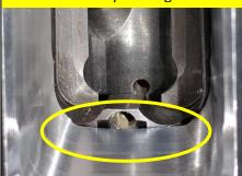
Align bedding bolts in chassis to holes in bottom of receiver. The rear bolt is under the trigger guard and can be accessed through a hole in the rear of the trigger guard.
